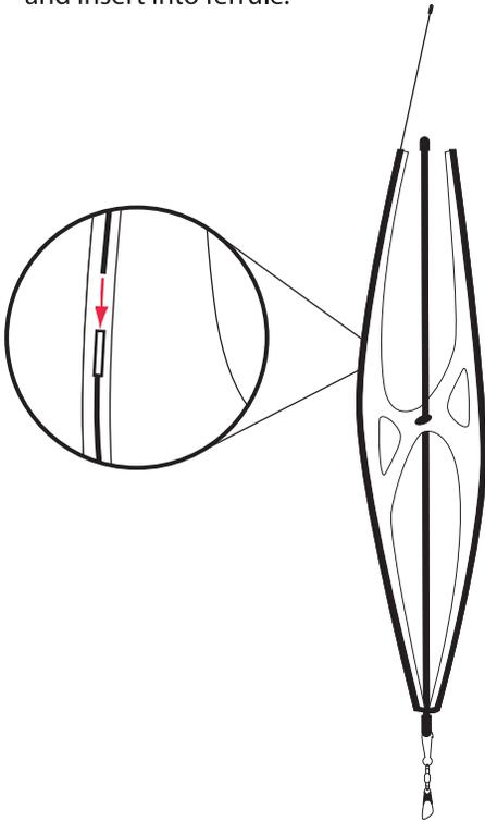
2. Slide the spar fully into the sail pocket and place tension cord into nock.
