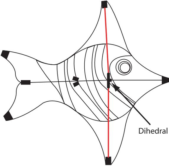
2. Insert one of the thicker spars with only one end cap, into the center dihedral connector and then into the pocket of the corresponding side. Repeat for the other side. Make sure that the dihedral is turned so the wings on the kite are swept away from the bridle
