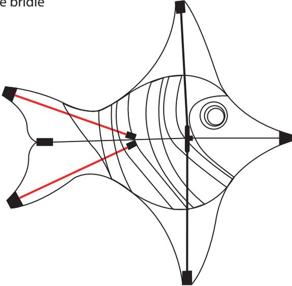
3. Then insert one of the spars with end caps on both ends, into the pockets located in the middle of the kite, and the other end into the tail pockets. Repeat for the other side.
