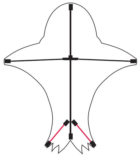
3. Insert the tail spar into the tail pockets in the seam.
