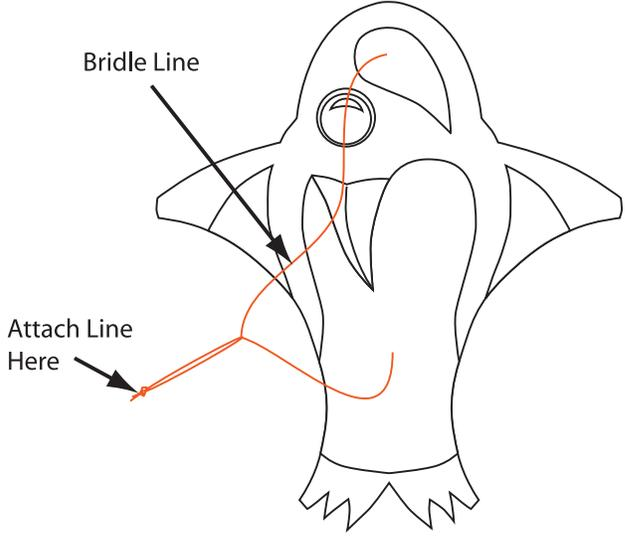
4. Finally, turn the kite over and attach line to bridle and fly!
