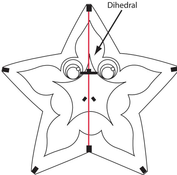
2. Insert a spar into the center dihedral connector and then into the pocket of the corresponding side. Repeat for the other side. Make sure that the dihedral is turned so the wings on the kite are swept away from the bridle
