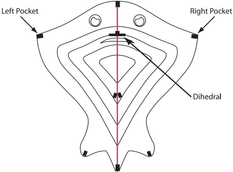
2. Insert a spar into the center dihedral connector and then into the pocket of the corresponding side. Repeat for the other side. Make sure that the dihedral is turned so the wings on the kite are swept away from the bridle.
